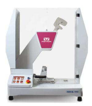
The Instron 9000 Series of pendulum impact testers are designed for determining the impact resilience of thermoplastics. Available in capacities from 0,5 to 50 Joules, the 9050 models are reliable and easy to operate.
