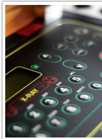
*This lightweight control unit is one of the two possible interface between any of the BALTOSPOT® pulsed wave generators and the operator.*
